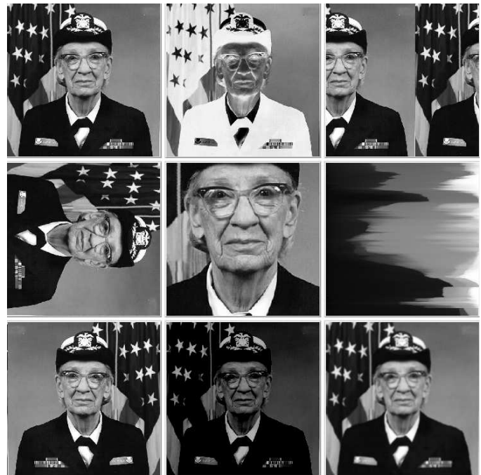
Figure 1: Example Image Processing Features. Top Row, from left: revert to original, make negative, scroll vertically by some number of pixels (200 in this example). Middle Row: Rotate 90 degrees, Zoom (center zoom chosen), Sort Rows by pixel value. Bottom Row: Flip Vertically, Darken Image, Blur Image. (Grace Hopper image from www.arlingtoncemetery.net/gopper.htm )
