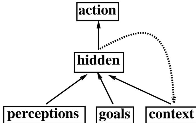
Figure 2.3: The initial architecture for the robot controller.
