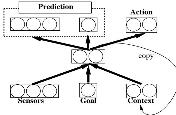
Figure 3.2: Control network used for one-dimensional environment.
