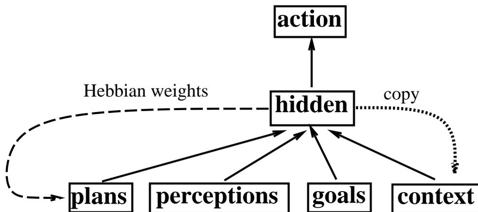
Figure 6.1: Architecture for storing protoplans for use within a single system.
