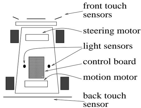
Figure 4.2: Positioning of sensors, motors, and control board on carbot.
