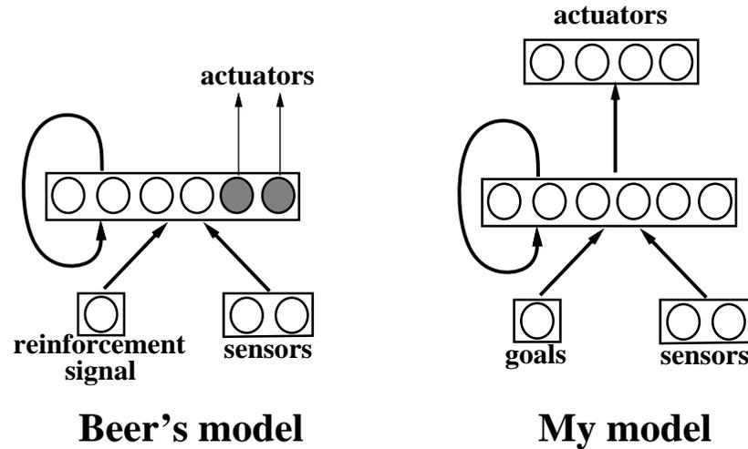
Figure 2.5: Comparing Beer's and my network architecture as applied to robotics control. Both versions contain a fully recurrent second layer of units. Beer's version does not contain an output layer per se. Instead certain units are designated for output (shaded here). In some of Beer's work, the second layer also receives input from a binary reinforcement signal.
