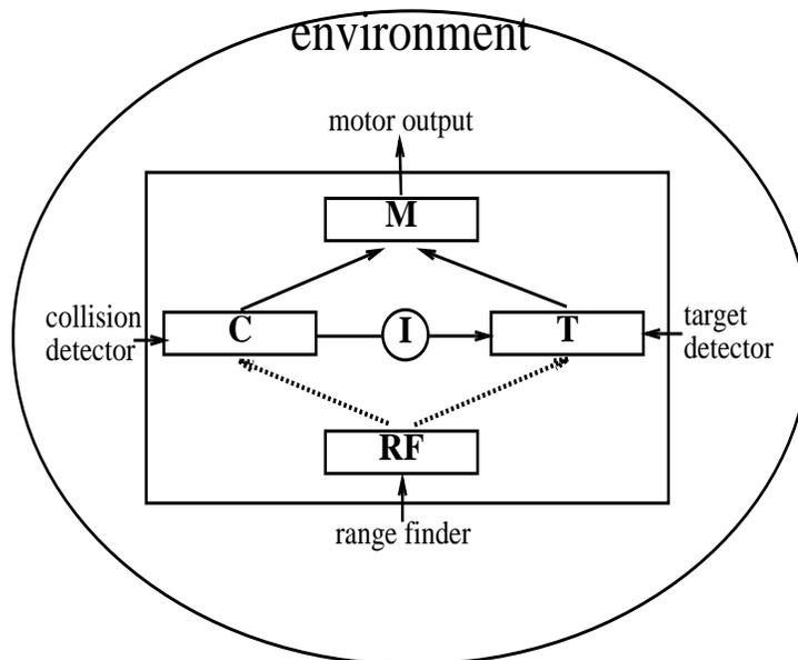
Figure 2.4: Schematic drawing of the distributed adaptive control architecture. Small rectangles depict groups of neurons. The solid lines represent prewired connections, while the dashed lines represent modifiable connections via Hebbian learning. There is an inhibitory unit (shown as **I**) between the collision detection and target detection groups to create a built-in preference for avoidance over approach.
