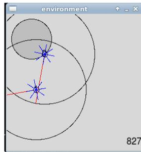
Figure 7: A robot locates a target area, and then begins to spin. When its front facing frequency sensor detects the other robot, the spinning robot emits a new frequency of 0.68.
