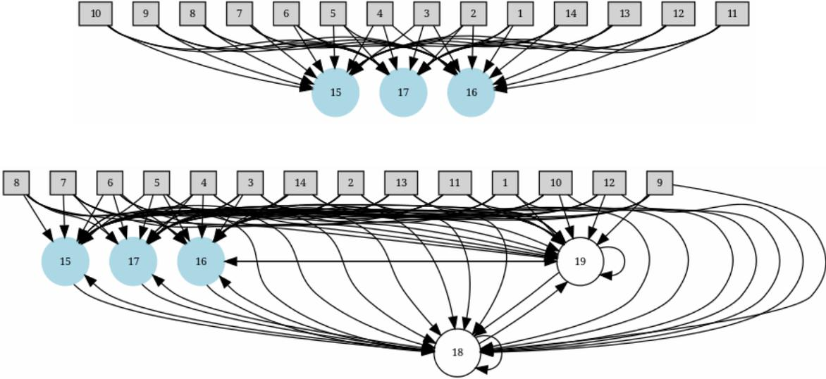
Figure 2: The feed-forward network with no hidden nodes (top) and the recurrent network with two hidden nodes (bottom). Inputs 1-8 are the sonar sensor values, inputs 9-12 are the four frequency sensors, input 13 is the target sensor, and input 14 is the robot’s own frequency emission.
