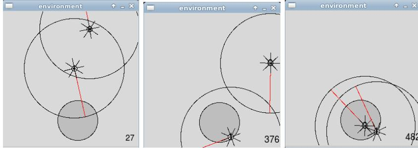
Figure 5: Our most successfully evolved neural controller, operating in our simplified environment. Three different situations arise based on what frequencies are heard and emitted (from left to right): avoidance, wall-following, and target cohabitation. The black circles indicate frequency range.
