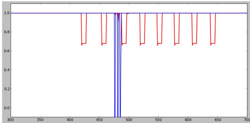
Figure 6: Robot 1 and Robot 2 explore the environment, both producing a frequency of 1.0. Robot 2 reaches the target and begins spinning, but does not change its frequency. Shortly after timestep 400, Robot 1 enters Robot 2s hearing range. While it is in range, Robot 2 emits a frequency around 0.68 whenever its front quadrant is facing Robot 2 (figure 7). This frequency does not seem to impact Robot 1s movement. Robot 1 does not find the target area continues past frequency range.
