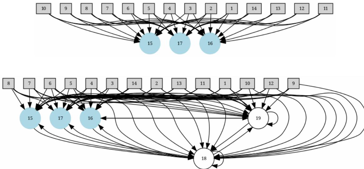
Figure 2: The feed-forward network with no hidden nodes (top) and the recurrent network with two hidden nodes (bottom). Inputs 1-8 are the sonar sensor values, inputs 9-12 are the four frequency sensors, input 13 is the target sensor, and input 14 is the robot’s own frequency emission.
