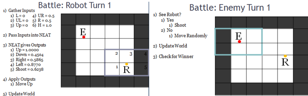
Figure 4: A round between the robot and the enemy. The inputs are gathered and passed into NEAT. NEAT gives the output and the maximum output is applied. The world is updated and the robot moves based on the implementation written. The world is updated once again and we search for a winner. This repeats until a unit dies or until 100 rounds have expired.
