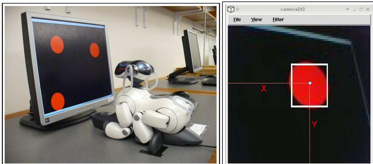
Figure 2: (Left) The “AIBO Television” experimental setup. The AIBO sits on a charger in front of a monitor that displays a graphics program. (Right) A sample AIBO camera image. The camera filter places a bounding box around red areas in the image. The sensory input for the robot is the  $x$ - and  $y$ - coordinates of the center of this bounding box.
