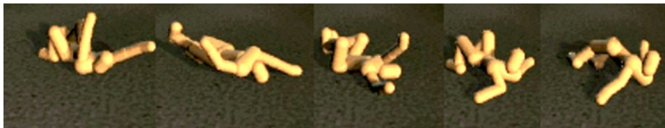
Figure 5: Crawling behavior from first run with fitness = \frac{distance}{energy+k}
