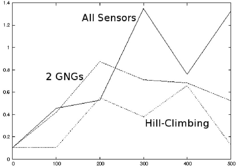
Figure 4: Graph showing the rate at which all three systems learned over the first 500 iterations. Note: maximum possible reward is 2.
