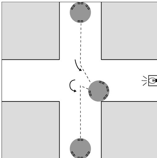
Figure 3: When learning with our original reward function (the sum of all light sensors), the Khepera maximized its reward not by moving to the light, but rather by getting stuck on a corner where it could see the light in three different sensors.
