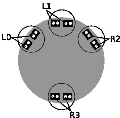
Figure 1: The Khepera’s 8 range and 8 light sensors (one of each per block) were grouped into 4 of each (L0-L3 and R0-R3).
