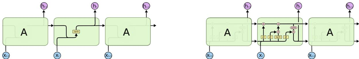
Figure 2: Left: The repeating module in a standard RNN contains a single layer. Right: The repeating module in an LSTM contains four interacting layers.
