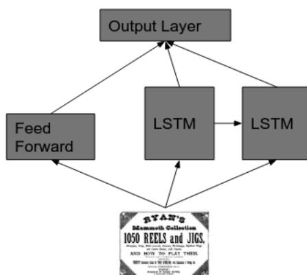
Figure 8: Potential network architecture which includes a feed forward layer as well as two LSTM layers one of which feeds into the other.
