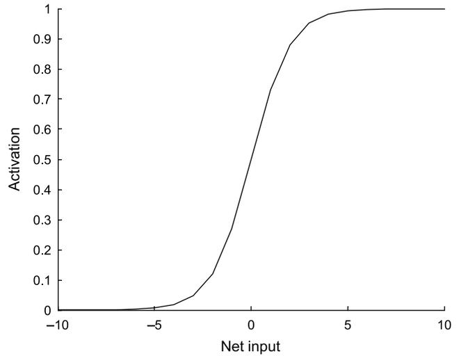
**Figure 2** Activation values as a function of net input for the asigmoid function.
