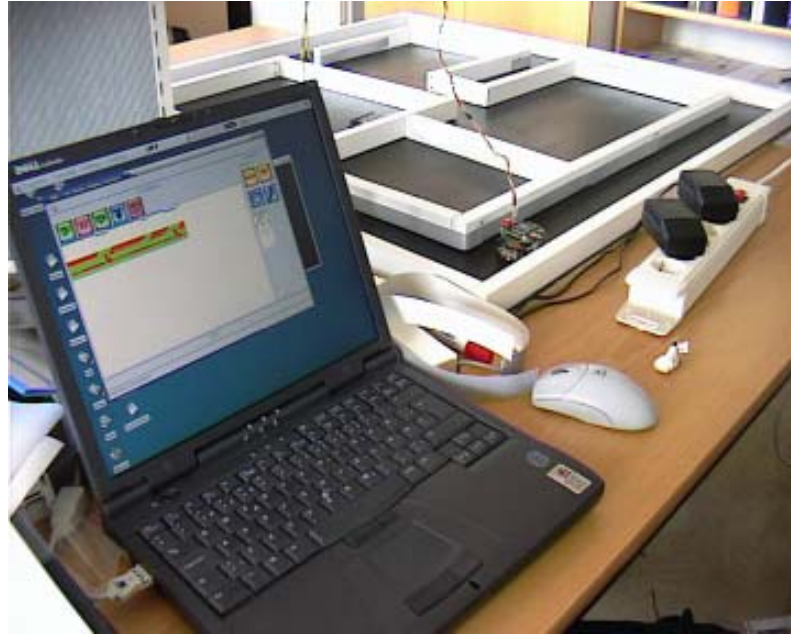
Figure 5.17: The real-world Khepera experiment setup with a laptop connected via a serial cable.
