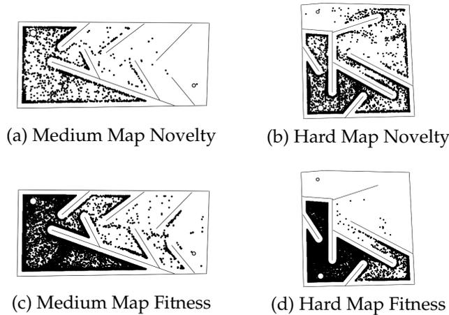
Figure 4: **Final Points Visited Over Typical Runs.** Each maze depicts a typical run, stopping at either 250,000 evaluations or when a solution is found. Each point represents the end location of a robot evaluated during the run. Novelty search is more evenly distributed because it is not deceived.
