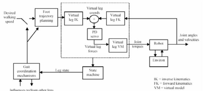
Figure 5: Control Diagram
