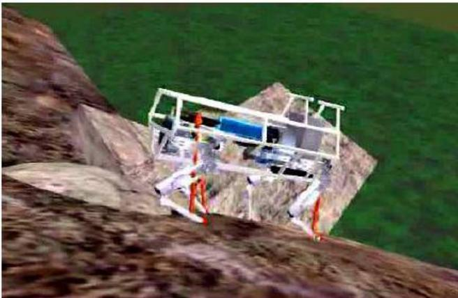
Figure 6: Image from physics-based simulation used to develop walking algorithms.
