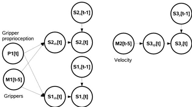
**Figure 8.** The most useful Bayesian network structures learnt for the gripper motor control (left) and the wheel velocity motor command (right). Both show that the motor commands affect the position of objects in the scene by changing their velocity. It has also learnt that the grippers’ touch sensor can be used to predict how the grippers move.
