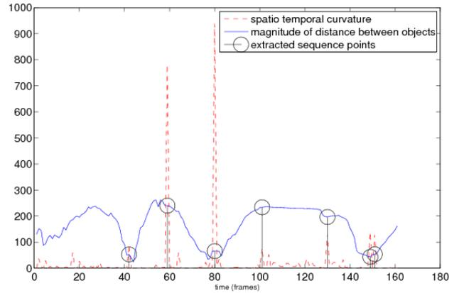
**Figure 10.** Extracting key points to imitate from an interaction sequence, shown in black circles. These points are extracted from peaks in the spatio-temporal curvature of the distance between the robot’s motor system and the object it wishes to interact with.
