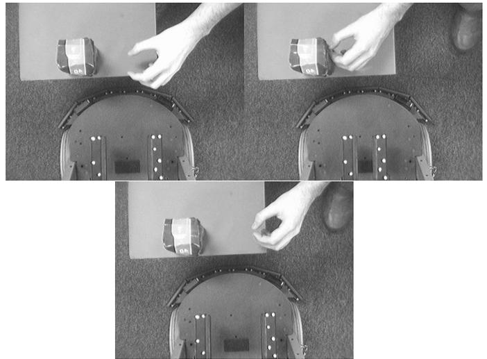
**Figure 11.** The first three sub-goals being imitated, extracted using the spatio-temporal curvature. Even though this action is occurring as the robot learns to control its gripper system, it is able to recognise it as an interesting action to imitate because neither the human hand nor the pack of biscuits can be accurately explained by its internal models.
