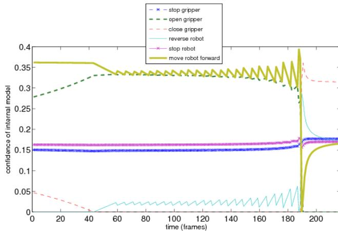
**Figure 13.** The progress of confidences of each learnt internal model in simulation as the robot tries to touch the object of interest. After this, the first goal state has been reached so the robot moves its grippers away to approach the next sub-goal.
