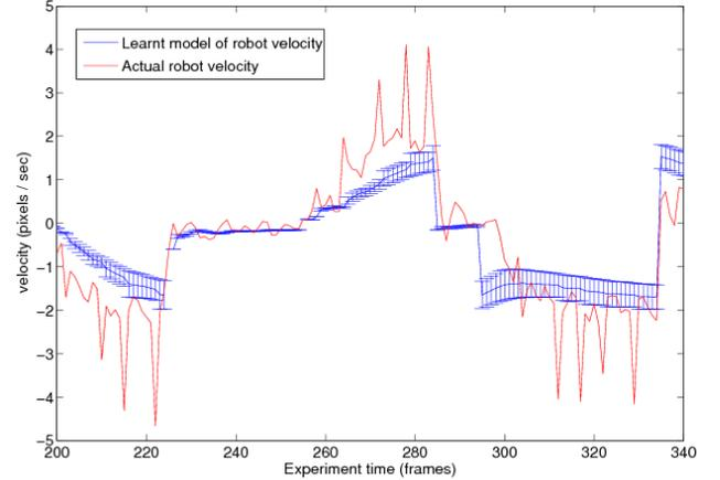
**Figure 6.** The robot learns online the mean and variance (shown with the error bars) of its velocity as it ‘babbles’ forwards and backwards. This is the prediction from the most accurate model, for which  $d=5$ . The large spikes in the actual data are because of dropped frames from the camera; the robot models this as noise.
