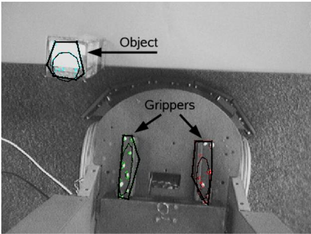
**Figure 3.** Moving image regions are clustered together; these regions are the robot's IOMs - internal models of where objects are in the scene. In this example, the grippers were moved by the robot, and the biscuit box object was shaken by a human demonstrator to make the robot aware of it. The thick black lines are the convex hull, and the thin ellipse shows represents the mean and covariance of the optical flow points' positions.
