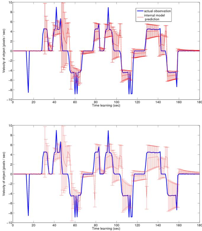
**Figure 7.** The predictions of two internal model structures for estimating the effect of the velocity motor command as the robot ‘babbles’ forwards and backwards. The top one can be seen to be the most accurate because it has the lowest estimated prediction variance, shown with the error bars. The structure of this model is shown in figure 8.
