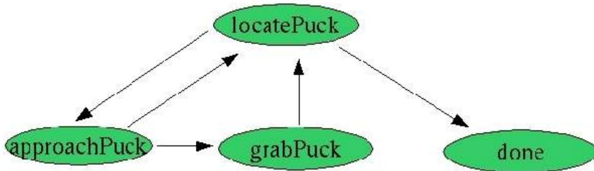
Example of FSM diagram for robot control to find and collect pucks
