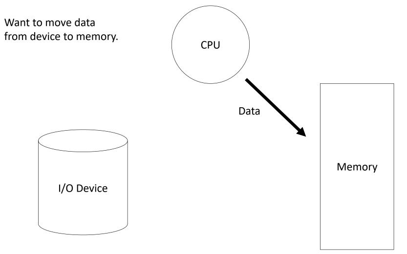
Want to move data from device to memory. CPU Memory I/O Device
