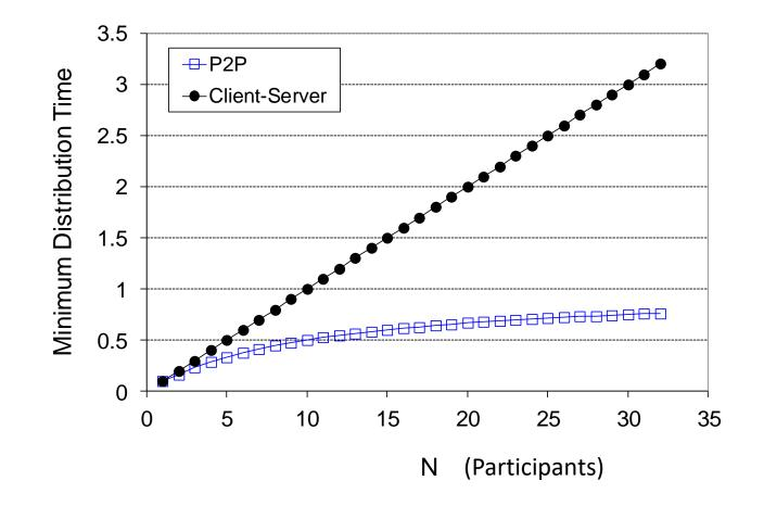
Let F = file size, client UL rate = u, server rate =  $u_s$ , d = client DL rate Assumptions: F/u = 1 hour,  $u_s = 10u$ ,  $d_{min} \ge u_s$
