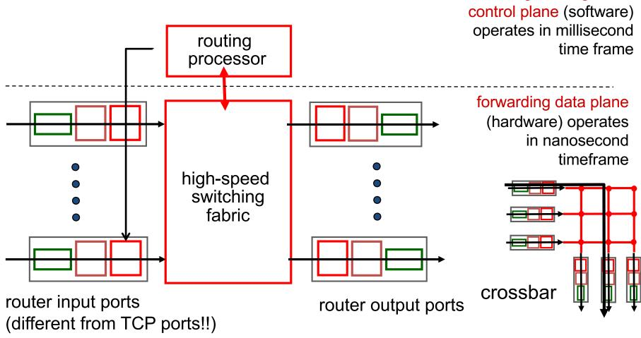
these are physical inputs/outputs to the router
