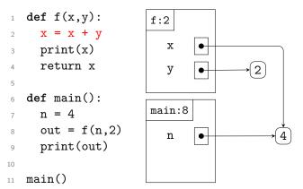
Once we've established the value of the arguments on line 8 (4 and 2, respectively), the f function is called. We create a new stack frame. Since f has two parameters, we create variables for them in the stack frame. They point to their corresponding values on the heap.
