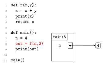
When line 7 of main is executed, the variable n is set to the value 4. We symbolize this by writing the variable name in the stack frame and creating an object on the heap for the value. We draw an arrow from the variable to its value.
