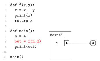
Once we've established the value of the arguments on line 8 (4 and 2, respectively), the f function is called. We create a new stack frame. Since f has two parameters, we create variables for them in the stack frame. They point to their corresponding values on the heap.
