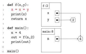
Note that the stack frame for main is keeping track of where we were in that function. When we are done with f, we will return to that line.
