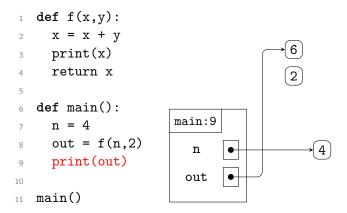
Line 4 will return the value of x to the place where f was called. As a result, the variable out in main is given the value 6, and the frame for f will be removed from the stack.
