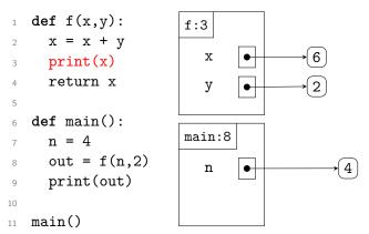
When we run line 2 in f, we will update the variable x by adding the contents of the variable y to it. Since ints are immutable, we will create a *new* object on the heap and make x point to it.
