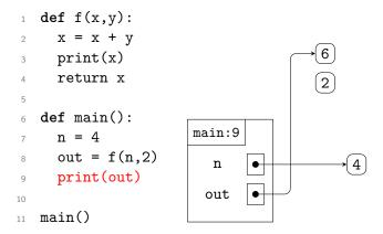
Line 9 prints the contents of the out variable (here, 6). After it runs, the main function is complete and the program is finished.
