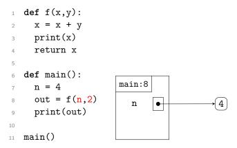
When line 8 is executed, we will call f. To do so, we must first determine the value of each of its arguments. In this case, the first parameter is n, whose value is currently 4. The second parameter is just 2.
