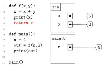
Line 4 will return the value of x to the place where f was called. As a result, the variable out in main is given the value 6, and the frame for f will be removed from the stack.
