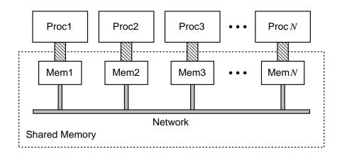
Figure 1 Distributed Shared Memory: Each processor sees a shared address space, denoted by the dashed outline, rather than a collection of distributed address spaces.
