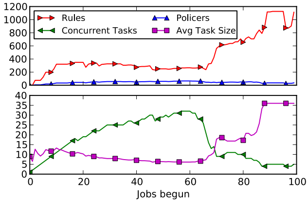
Figure 6: Rule and policer count, along with the number and average size of concurrently executing tenant tasks for a switch during the Squid Mean = 150, Oversub = 5 run described in Figure 4.
