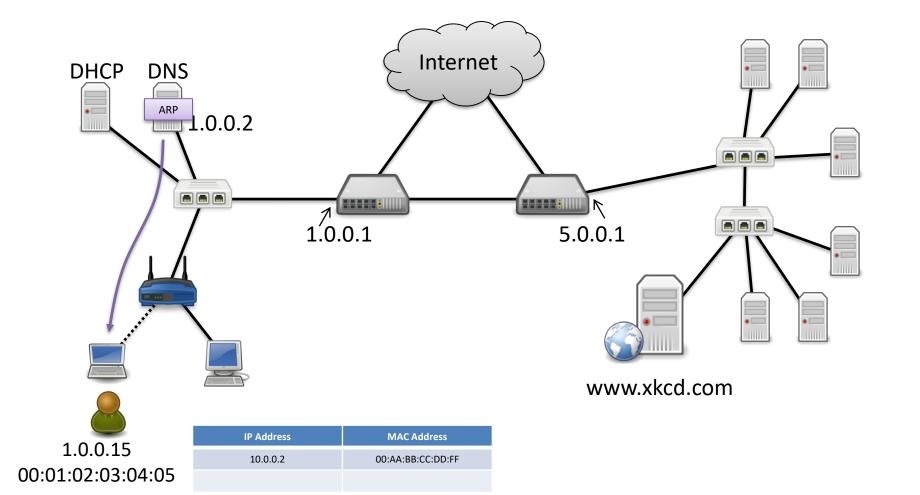
User queries local DNS resolver for www.xkcd.com. Resolver runs necessary queries (root, TLD, etc.)
