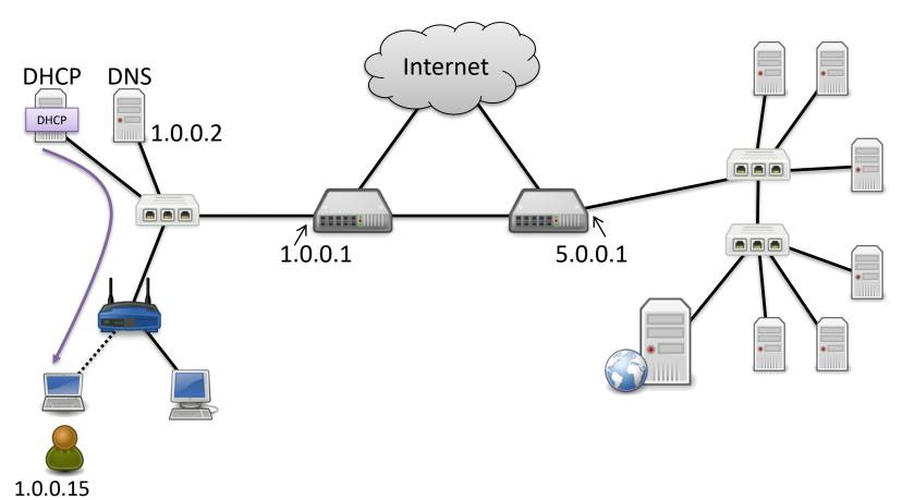
Suppose user tries to access website: www.xkcd.com Must resolve name using DNS. Query local resolver.
