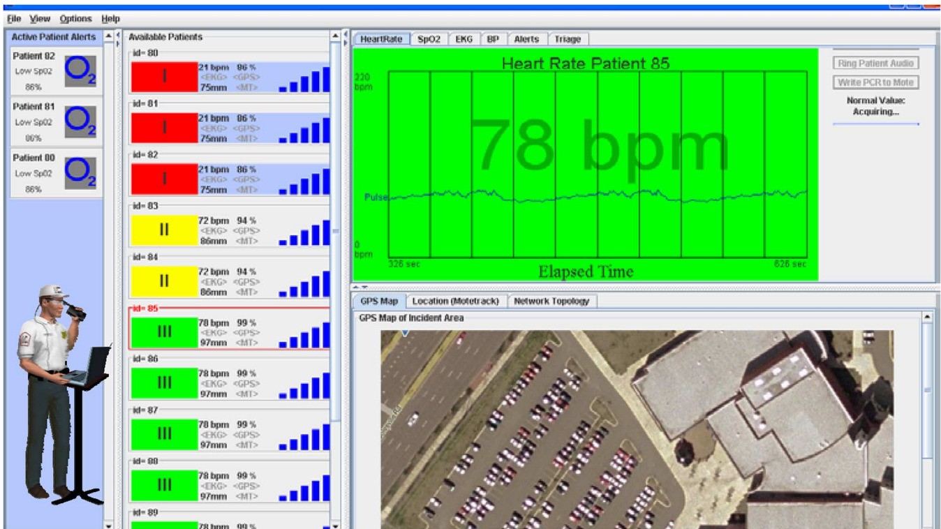
Fig. 6. Graphical user interface on the general purpose personal server that monitors the vital signs at a mass casualty incident.
