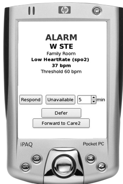
Figure 6. Caregiver's view of an alarm. Clicking on "Respond" indicates that the caregiver will handle the alarm.
